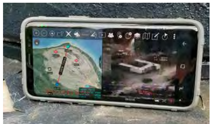
An Android Tactical Awareness Kit shows location data and an image feed during Northern Strike 20, at Rogers City, Michigan. Joint Terminal Attack Controllers regularly use the ATAKs to see location of forces and coordinate close air support.
